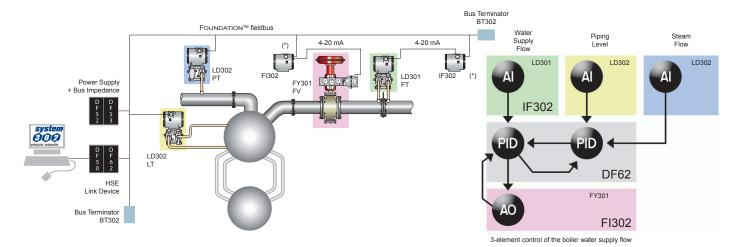
$^{\ast}$  external sources powering the 4-20mA equipment were suppressed to simplify the design.
