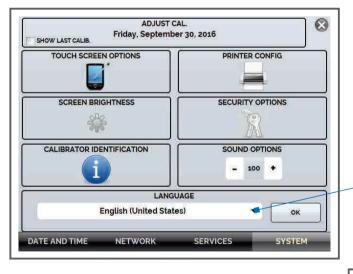
We provide a protected access to the calibration menu of the TA, so that you can send it to any good calibration laboratory in case an adjustment is needed.
