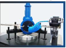
With flange adapters, clamps and bubble jar (API 527)
