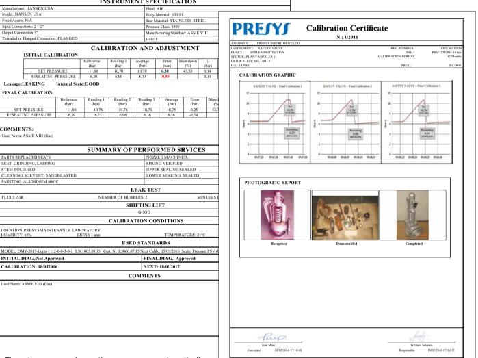
The set pressure and reseating pressure are automatically registered and display on the digital pressure registration system and can be send in real-time to the ISOPLAN® Software.
