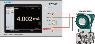
Current input with high accuracy, allowing the instrument *TRIM* and *loop test*.
