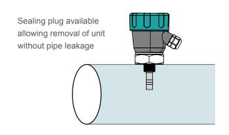
High level switch in grain application
