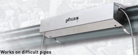
The WD Series is available with three transducer types and is suitable for inner diameters ranging from 50...6500 mm. The strong signal output and noise suppression technology make it possible to use the WD Series on all pipe materials, even on such challenging ones as fiber-reinforced plastic (FRP) pipes. The outstanding performance of FLEXIM is shown by thousands of references worldwide. Contact your local FLEXIM support office for more details.
