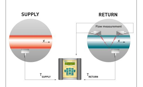
FLUXUS<sup>®</sup> F601 Energy measures the thermal energy consumed by a system by determining the heat or cold flows entering and exiting it (difference method). For doing so, temperature measurements at the supply and return lines as well as the measurement of the volume flow through the system are required. FLUXUS<sup>®</sup> uses the measured values to calculate the thermal energy flow based on the heat transfer media's enthalpy curves stored in the internal memory.
